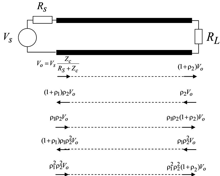
$$\rho_1 = \frac{R_s - Z_c}{R_s + Z_c} = 0.5 \quad \rho_2 = \frac{R_L - Z_c}{R_L + Z_c} = -0.25$$
